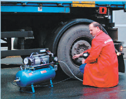
Filling of tyres with 16-bar pressure.
